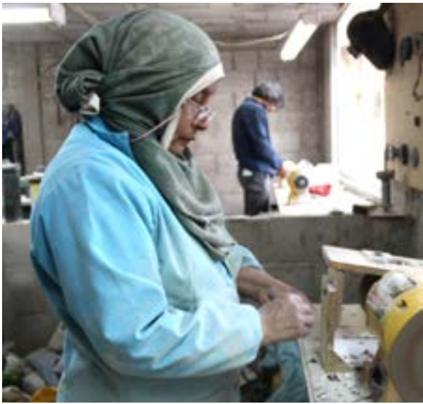
Magdalena uses a cotton buffing wheel buffer to polish the best selling earrings bearing her name.
